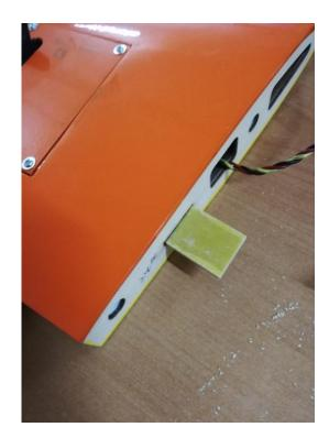
Glue the fiberglass' 2,5cm part on the wing. Use sandpaper on the fiberglas for better glue result.
