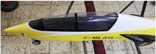
Cut the canopy to fix, while the base part screwed on the fuselage. Use Patex soft glue (or similar). Also use 8pcs 2,5 x 12mm screws - included in the kit.
