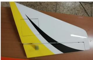
Cut the oracover for flap hinges and use epoxy glue. Use sandpaper on the horn parts for better glue result.
