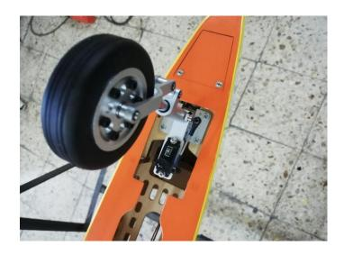
Stick the plastic pools to the mid-wing with epoxy glue, than screw the retracts with 12pcs 3 x 20mm screws included in the kit.
