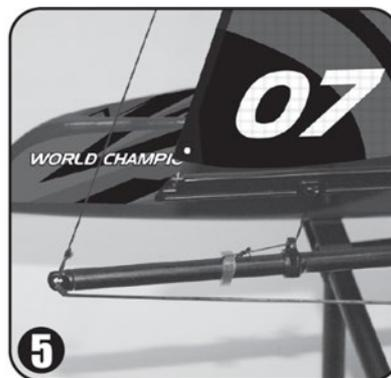
6. Use jib boom cord to thread through the second boom bend eye (from front side back to rear side) located in central spar, thread through the sheeting deck eyelet on forward cross beam, attach cord loop to the pin as picture shown.
