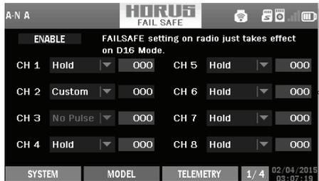
3. Failsafe can be set on receiver via short press F/S button while moving channel position to a preset value after binding.
